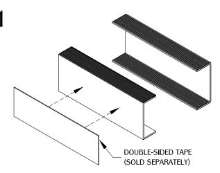
Detach front portion of the WM1 from the back. Apply adhesive or double-sided tape to the back side of the WM1 accordingly. If purchased with pre-installed double-sided tape, proceed to step 2.
