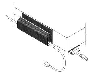
Apply pressure to the WM2 when placing against the work surface until it is held into position by the adhesive.
