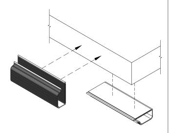
Apply adhesive or double-sided tape to the back of the WM2. If purchased with double-sided tape pre-installed, proceed to step  $2. \,$
