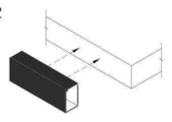
Apply adhesive or double-sided tape to the back of the WM3. If purchased with double-sided tape pre-installed, proceed to step 2.
