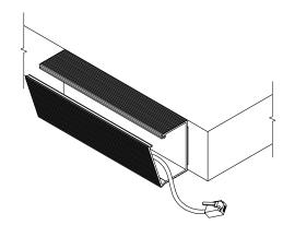
Pop open the WM3 so that wires may be placed inside using the opening on top of the unit.
