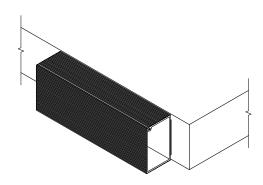
Apply pressure to the WM3 when placing against the work surface until it is held into position by the adhesive.
