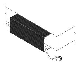
After placing wires inside the WM3, snap the unit back into the closed position.
