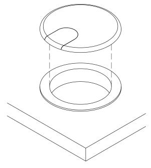
Install XG1 into the cut out and be sure it is fully leveled onto worksurface.
