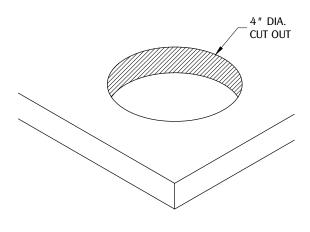
Make a cut out on the desired surface. (<u>Note</u>: We do not recommend cutting before receiving part or part sample.)
