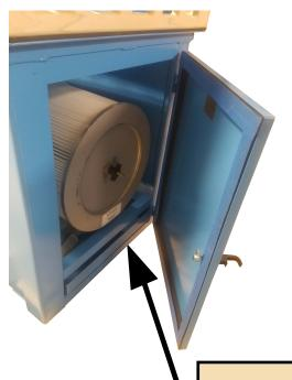
The filters will clean better with machine off, you may shut machine off and before it slows down to a complete stop, pulse the filter and allow the fan to prevent the dust from exiting the filter compartment.
