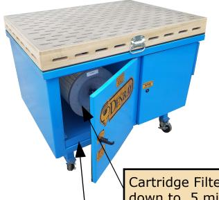
The filters will clean better with the machine off. You may shut the machine off and before it slows down to a complete stop, pulse the filter and allow the fan to prevent the dust from exiting the filter compartment. Filter replacement number is on the gold sticker on the outside of the machine. Be sure to replace with same type of filter or a filter made of polyester media.
