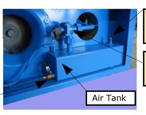
150 psi Pressure, relief valve 1/4" Male pipe thread
