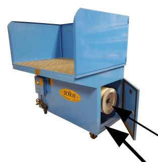
The filters will clean better with machine off, you may shut machine off and before it slows down to a complete stop, pulse the filter and allow the fan to prevent the dust from exiting the filter compartment. Filter replacement number is on the inside of the filter door. Be sure to replace with same type of filter or a filter made of polyester media.
