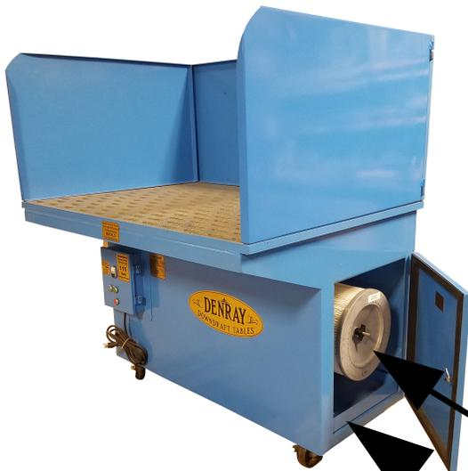
The filters will clean better with machine off, you may shut machine off and before it slows down to a complete stop, pulse the filter and allow the fan to prevent the dust from exiting the filter compartment. Filter replacement number is on the inside of the filter door. Be sure to replace with same type of filter or a filter made of polyester media.
