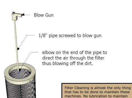
The cleaner the filters are kept the better the machine will perform. The dirtier the filters the harder it is to
