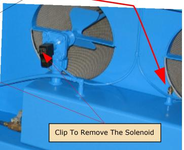
Solenoid to activate the valve 120 Volts
