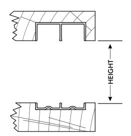
Use glue or brads to fasten track and guide to mounting surface.
