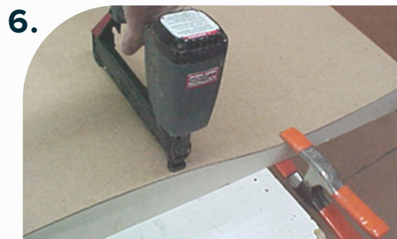
Staples can be applied along framework for extra reinforcement.
