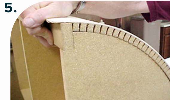
Press pre-sized and pre-cut panel to framework.
