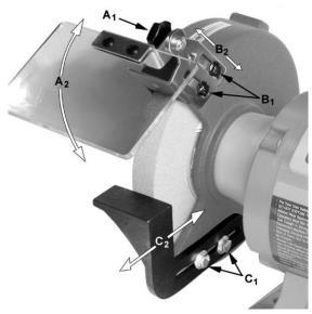
Figure 8-1: eye shield adjustment
