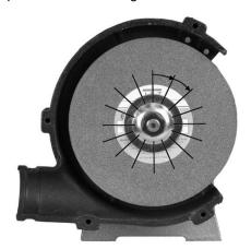
Figure 9-2: wheel balancing
