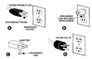
Figure 7-1: plug configurations
