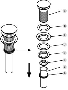
Begin by removing the nut (h), tailpiece (g), mounting nut (e), plastic washer (d) and concave washer (c)
