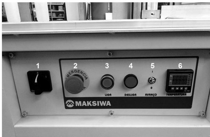
1. Turn the main switch (1). This key energizes the machine's panel, without turning it on.
