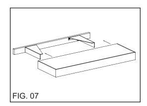
**Step 8:** When you are satisfied that the *Floating Shelf* is located correctly, screw or pin the *Floating Shelf* to the *Wood Mounting Plate* as shown. Drill two 1/8 inch pilot holes in the *Floating Shelf* at the locations shown in figure 08 when using the two #6 x 3/4 inch Flat Head Screws provided.
