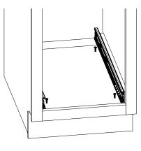
Step3: Reinstall Tray Roll-Out onto support sled.
