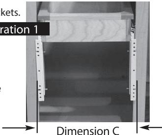
**Step 2:** Measure the distance from the bottom face frame to bottom of the Door Bracket. Note as Dimension A. Measure your door overlap. Note as Dimension B. (See illustration 2) Note: On frameless cabinets, measure from the bottom of the cabinet opening to the bottom of the Door Bracket.
