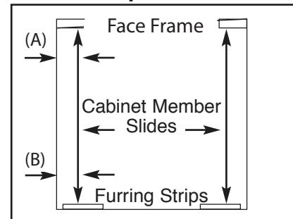
**Step 5:** Mount Rear Bracket. Extend the slide rear mounting bracket until it contacts the rear (Furring Strip). Bottom of slide should be  $7\frac{3}{4}$ " from cabinet floor. Rear mounting bracket should be the same distance from the side cabinet wall at rear of slide as it is up front. Drive mounting screw in center horizontal slot of rear mounting bracket, tighten. Tighten screw in front bracket.
