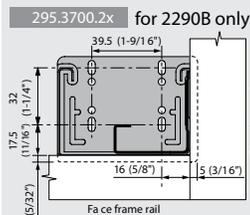
NOTE: For frame applications. Minimum 3 screws per bracket.
