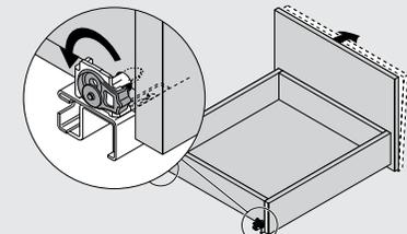
Tool free tilt adjustment +5 mm.
