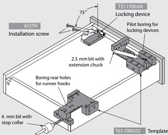
Important: Use of the T65.1000.02 template is recommended for accurate location and angle of locking device pilot holes.
