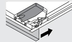
1. Place drawer on runners and close, locking devices will automatically connect to runners
