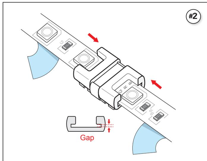
Insert FlexTape® into slots on both ends until fully seated
