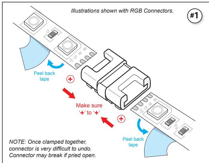
Peel back FlexTape® backing. Be sure to match polarity (+ to +)
