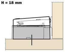
$\ensuremath{\textbf{1}}$  - Loosen one of the two fixing screws of the mounting plate.
