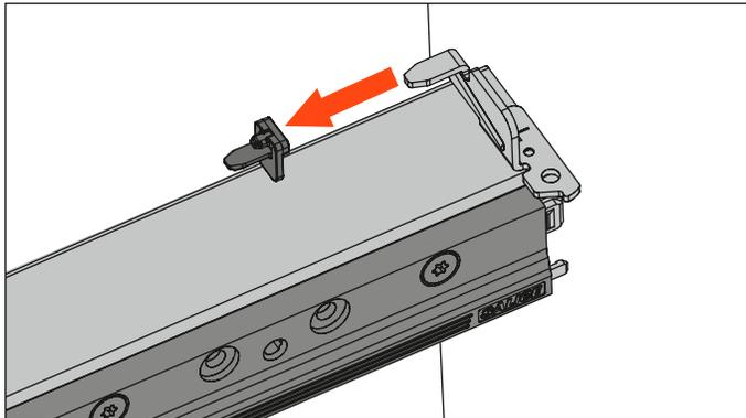
Insert the tilt adjustment levers, both right and left.
