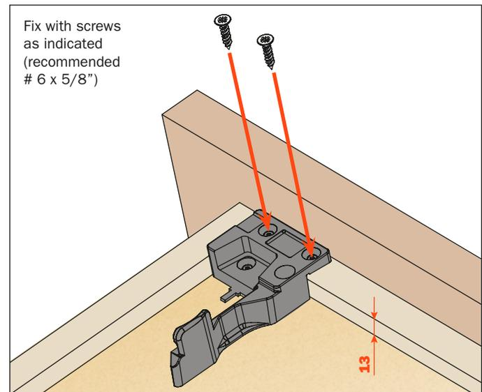
Use **drilling template** for accurate installation of the clips, see page 60.
