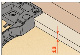
Height of the sub front must be 13 mm (1/2").
