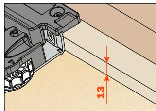
Use **drilling templates** for accurate installation of the clips, see page 60.
