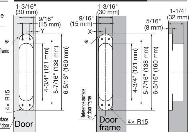
\* When using the optional square screw cover, drill the first oval hole (surface hole) in both the door and the frame as a square hole of width width 1-3/16" (30 mm) x length 6-5/16" (160 mm) x depth 5/16" (8 mm)
