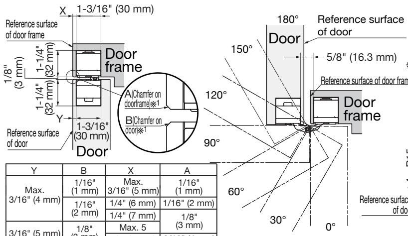
\*1 Chamfer is needed depending on the amount of X and Y.
