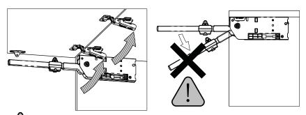
When installing the door, do not bend the arm down as it may spring back violently and cause injury.
