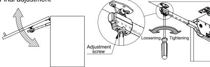
· If you feel that the door is too light (self lift-up) or too heavy (self-closing), it is possible to limit the action of the spring by tightening the adjustment screw.
