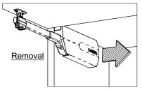
To remove cover, pull the back side first.
