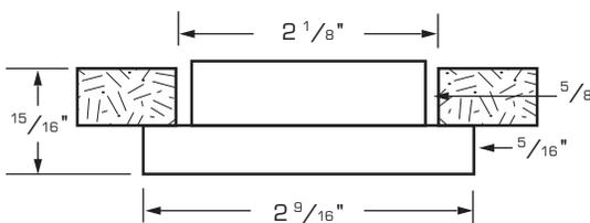
cross section for surface mounting
