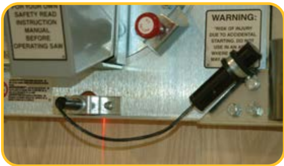
An optional laser line provides a better view of your cutting line
