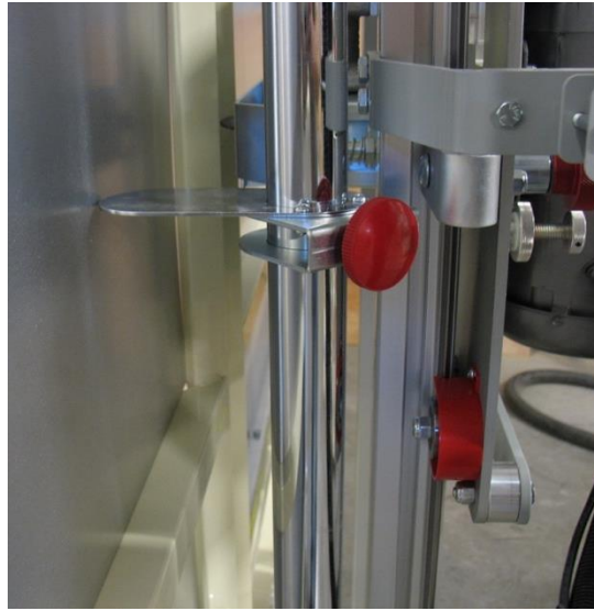
Figure 30: Kerf Spreader, in-line with saw blade, operational position
