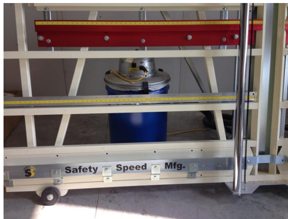
Fig. 62: Midway fence installed
