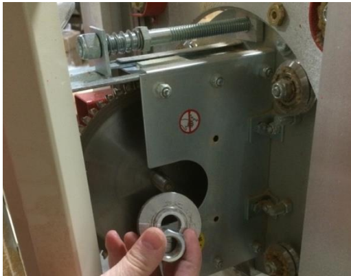
Figure 24: Outer Blade Flange & Arbor Nut Removal
