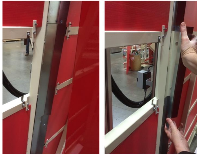
Figure 18, A & B: Removing Center Frame Filler Insert (7000HD shown)
