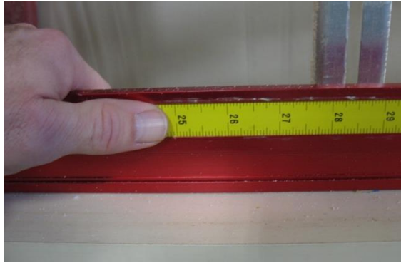
Figure 27: Crosscut Ruler Adjustment
