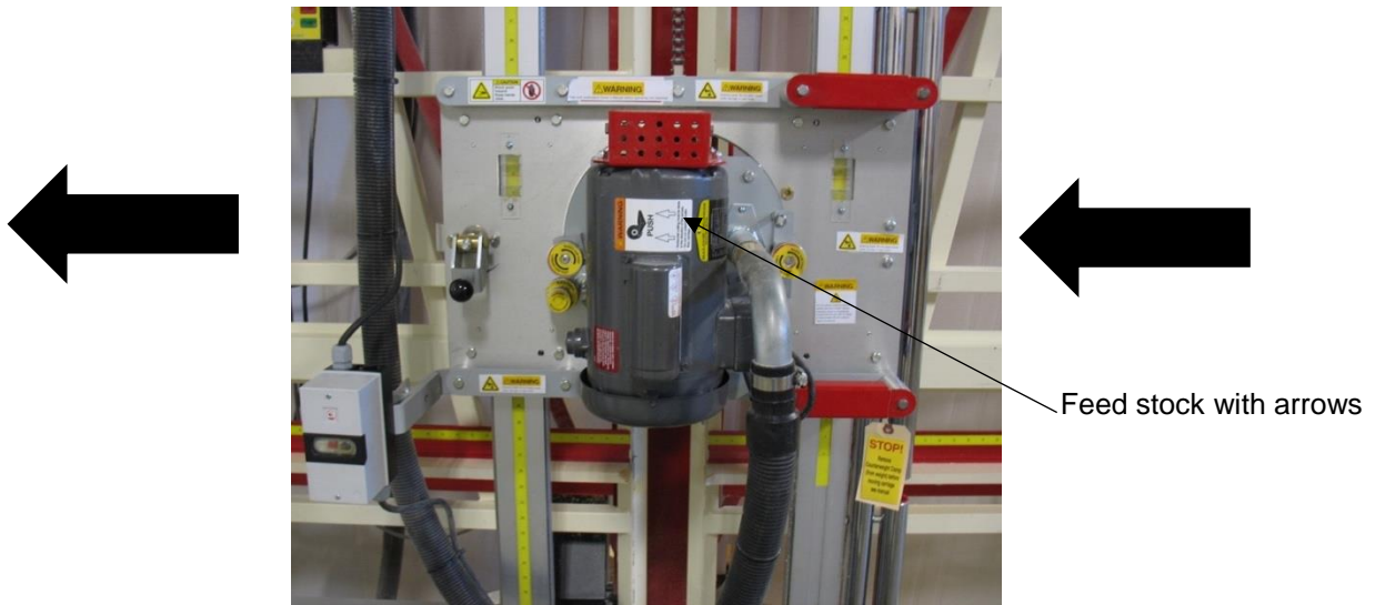
Figure 48: Rip cutting motor position (7400 shown)
