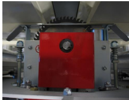
Figure 50: Saw Foot (guard & chatter preventer) in position for rip cutting (7000 shown, top-down view)
