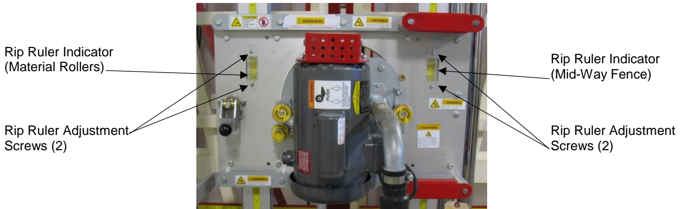
Figure 28: Rip Cut Ruler Adjustment (Rip Position, 7400 shown)
