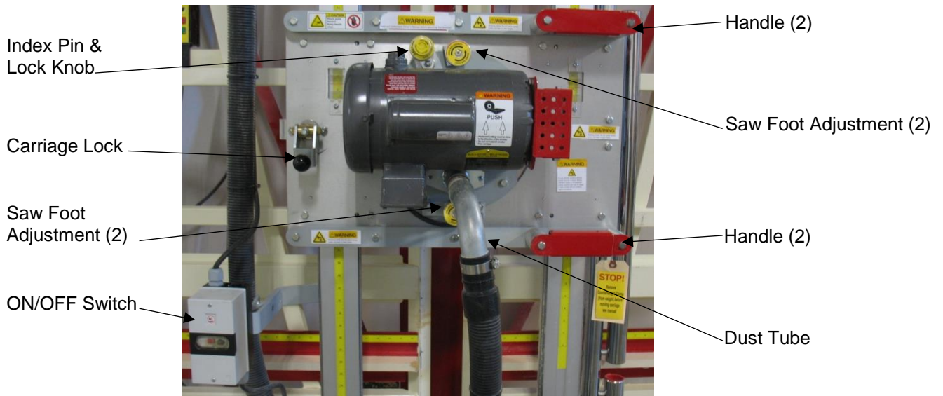
Figure 40: Basic Operating Controls and Components, 7400 shown
