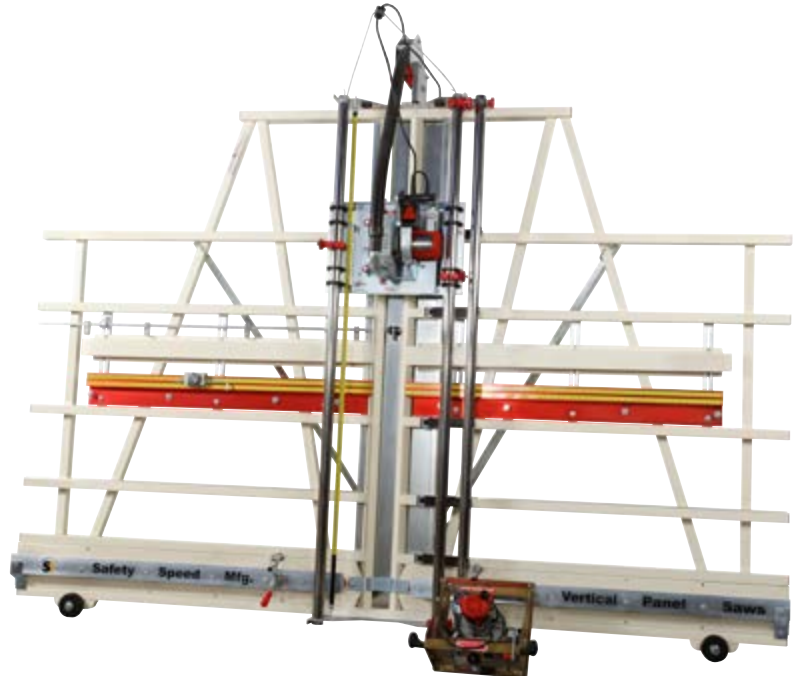
This photo is shown with a stand, wheels, hold down bar and a dust kit which are optional accessories
