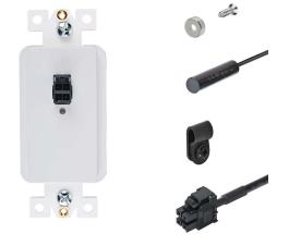
Docking Drawer's Safety Interlock Disconnect Kit with Magnetic Limit Switch enhances the safety of stationary kitchen appliance garages by powering off the outlet and up to 4 connected devices whenever the cabinet door is closed. This safety outlet can be wired in-series with the included receptacles, featuring (4) 20amp AC ports. ETL Listed to UL 498 and CSA 22.2 #42 and approved for use in the US & Canada\*. Possible applications include:
