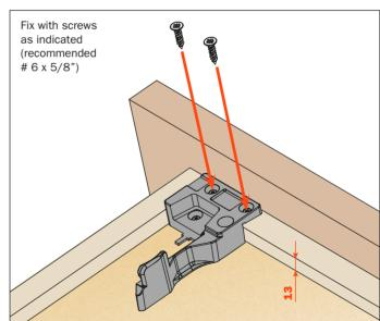
Use **drilling template** for accurate installation of the clips, see page 62.
