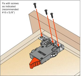
Use **drilling templates** for accurate installation of the clips, see page 62.
