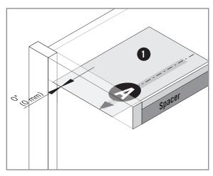
For faceframe installation a spacer needs to be installed at the cabinet ceiling so the installation level is flush with the face frame.
