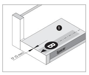
For faceframe installation a spacer needs to be installed at the cabinet floor so the installation level is flush with the face frame.
